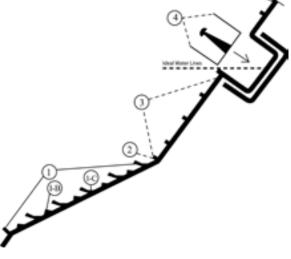
(Area 2) This is the riffle transition and large nugget recovery area. Nuggets too large to spiral up the riffle in area (3) into concentrate cup (4) will remain in area (2) until visually sighted and removed.
