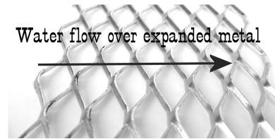
When you are replacing the expanded metal in your sluice after a cleanup it is important to orient the expanded metal properly. One edge of each expanded diamond acts exactly like a miniature riffle trapping gold behind the riffle. If you put the expanded metal piece in backwards this riffle effect is lost, and the expanded aluminum will only act to catch stones and make cleanup more difficult. The correct orientation of the expanded metal is illustrated above.
