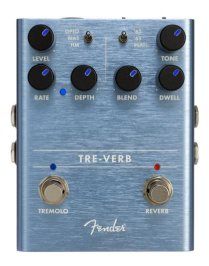
Tremolo and reverb pedal Independent Tremolo and Reverb effects with three voices each Tap Tempo for Tremolo rate Stereo inputs and outputs LED-backlit knobs
