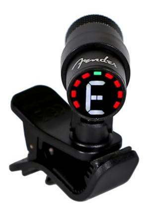
Built with live performance reliability and aesthetic in mind, the Bullet Tuner provides a nonintrusive, staunchly accurate tool for musicians at every stage. A powerful engine with a noise-proof vibration sensor allows for precise chromatic tuning for electric, acoustic and bass guitar players alike—while a bright, color LED screen shows easy-to-see readings in any environment.
