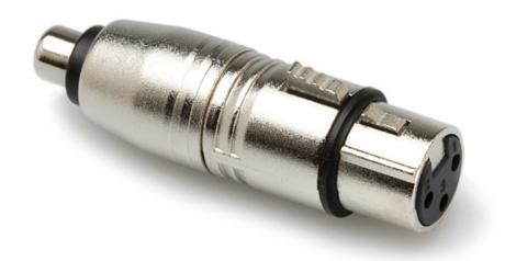
Hosa GXF-132 RCA Female to XLR Female. This adaptor is designed to adapt a phono plug to an XLR output. XLR pin 3 is grounded resulting in an unbalanced signal.
