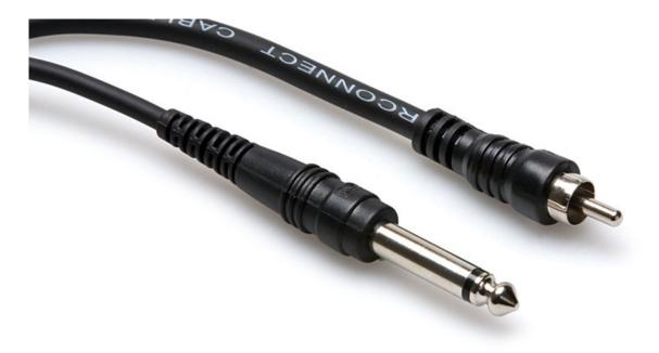
Hosa CPR-105 RCA Male to  $1/4^{\prime\prime}$  Phone Male with Molded Plugs. This cable is designed connect gear with unbalanced phone jacks to gear with phono jacks. It is ideal for connecting pro audio gear to consumer audio components.
