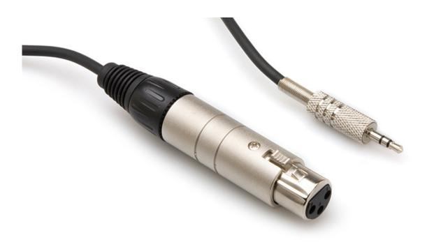
Hosa MIT-156 Line Matching Transformer. 600ohm Low-Z to 2500ohm Medium-Z. This adaptor is designed to match 600R output impedance to 2.5K input impedance. It may be used to connect a microphone to a portable recording device, camcorder, or PC.
