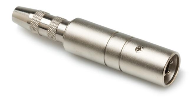
Hosa MIT-129 1/4" Female Hi-Z to XLR Male Lo-Z. This adaptor is designed to match 50K output impedance to 200R input impedance. It is ideal for connecting a hi-Z instrument to a microphone input. Every acoustic guitarist and bass player should keep one of these in there instrument case.
