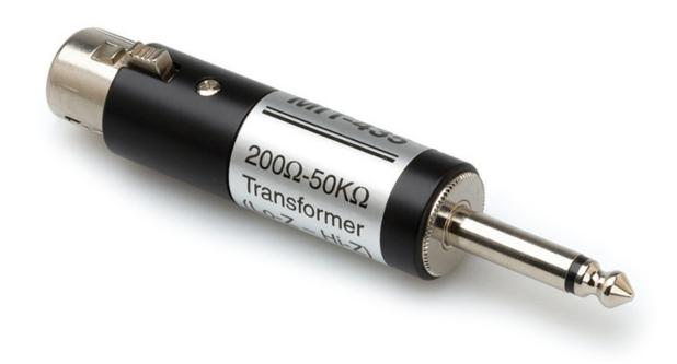
Hosa MIT-435 XLR Female Lo-Z to 1/4" Male Hi-Z. 200ohm Low-Z to 50Kohm High-Z. This adaptor is designed to match 200R output impedance to 50K input impedance. It is ideal for connecting a microphone to hi-Z instrument jack.
