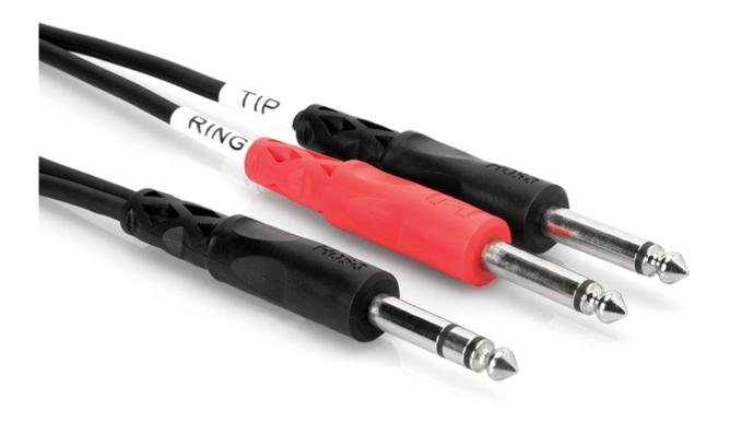
Hosa STP-202 Single  $1/4^{\prime\prime}$  TRS to Two  $1/4^{\prime\prime}$  TS. This cable is designed to connect a channel insert on a mixing console to an effects processor with unbalanced phone jacks. Leads are labeled TIP (send) and RING (return) to aid in identification.
