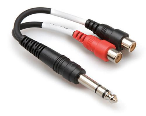
Hosa YPR-102 Stereo 1/4" Male to Two RCA Females. This cable is designed to split a stereo signal. Black- and red-coded phono jacks indicate left and right respectively. It may also be used in reverse.
