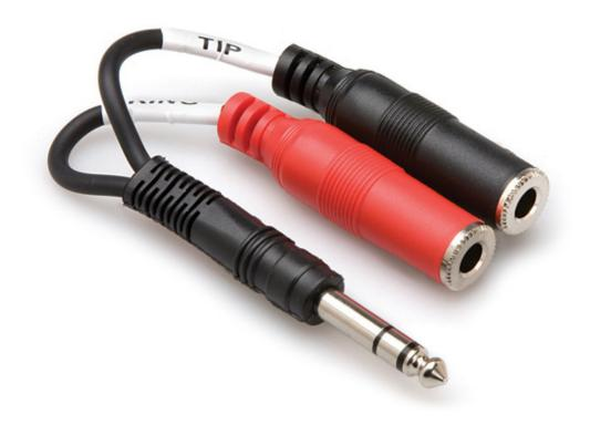
Hosa YPP-117 Stereo 1/4" Male to Two Mono 1/4" Females. This cable is designed to split a stereo signal. Black- and red-coded mono phone jacks indicate left and right respectively. It may also be used to adapt a stereo cable with mono phone plugs to a stereo phone jack.
