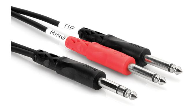
Hosa STP-204 Single  $1/4^{\prime\prime}$  TRS to Two  $1/4^{\prime\prime}$  TS. This cable is designed to connect a channel insert on a mixing console to an effects processor with unbalanced phone jacks. Leads are labeled TIP (send) and RING (return) to aid in identification.
