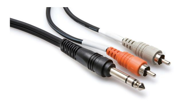
Hosa TRS-204 Single 1/4" TRS to Two RCA. This cable is designed to connect a channel insert on a mixing console to an effects processor with phono jacks. Leads are labeled TIP (send) and RING (return) to aid in identification.
