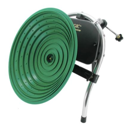
Gold Magic 12-10 Spiral Panning Machine. This gold wheel does not require pre-classification. It can be used to process raw material.
