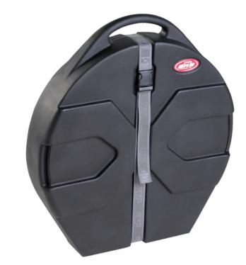
Roto molded of Linear Low Density Polyethylene with a welded center post that will hold seven or more cymbals\* this cymbal case has become the drummer's choice. Complete with four cymbal pads and a storage pocket, the cymbals will travel without pressure on the sound edge. Molded with the "X" pattern this redesigned Cymbal Vault will stack conveniently with the SKB Roto-X Drum Cases.
