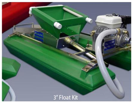
A Proline float kits allow you to work in deeper water with the advantages of a conventional dredge. This is Proline's floatation kit that is available for the 3" dredge/highbanker combo.
