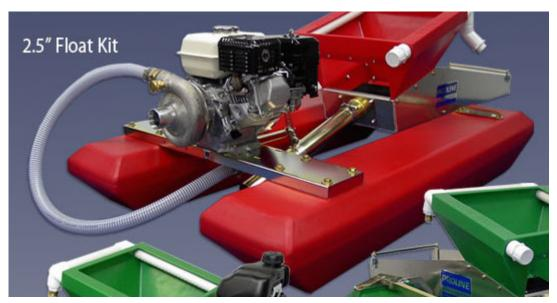
A Proline float kits allow you to work in deeper water with the advantages of a conventional dredge. This is Proline's floatation kit that is available for the 2.5" dredge/highbanker combo.
