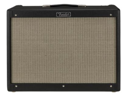
40 watts; Normal, Drive, and More Drive channels Celestion 12" A-Type speaker Modified preamp circuitry for increased overdriven note definition Spring reverb modified for improved smoothness Lightweight pine cabinet Includes 2-button footswitch and cover
