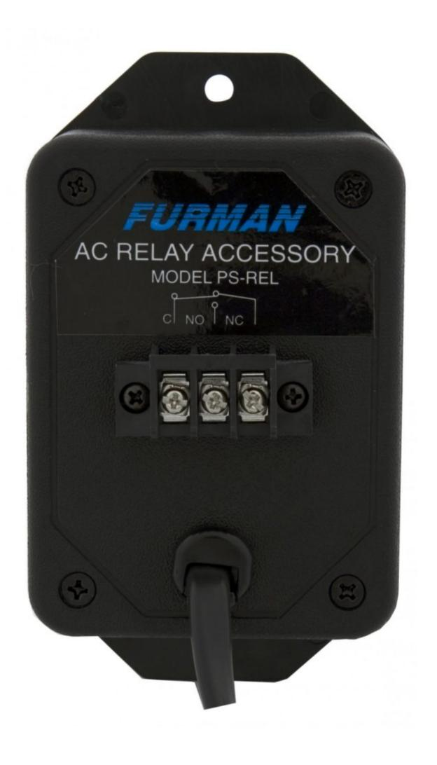
The PS-REL AC Relay provides an alternate way of closing switch contacts. Instead of being operated manually like the RS-1, it is a relay that detects the presence of AC power and, in response, closes relay contacts that are wired to a terminal strip. It may be used with any of the Furman products mentioned in connection with the RS-1.
