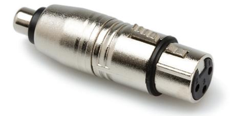
Hosa GXF-132 RCA Female to XLR Female. This adaptor is designed to adapt a phono plug to an XLR output. XLR pin 3 is grounded resulting in an unbalanced signal.
