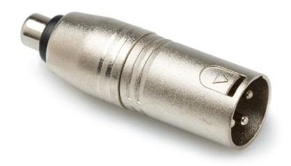
Hosa GXM-133 RCA Female to XLR Male. This adaptor is designed to adapt a phono plug to an XLR input. XLR pin 3 is grounded resulting in an unbalanced signal.
