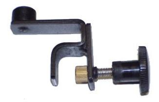
A "C" clamp style that mounts to drum rims or tension rods. Fits mounting surfaces up tp 7/16" thick and provides the standard 5/8"-27 thread mic mount.
