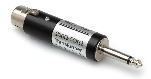
Hosa MIT-435 XLR Female Lo-Z to 1/4" Male Hi-Z. 200ohm Low-Z to 50Kohm High-Z. This adaptor is designed to match 200R output impedance to 50K input impedance. It is ideal for connecting a microphone to hi-Z instrument jack.
