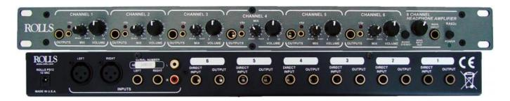
The ROLLS RA62c is a six-channel headphone/earphone amplifier for professional audio monitoring. A variety of input options are available including 1/4", RCA, and balanced XLR. Since the MONO/STEREO switch is after the pan control, it will mix 2 MONO signals and their balance can be adjusted with the Pan control. With the addition of rear panel Direct Input connectors, each channel may mix a second stereo signal.
