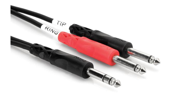
Hosa STP-202 Single 1/4" TRS to Two 1/4" TS. This cable is designed to connect a channel insert on a mixing console to an effects processor with unbalanced phone jacks. Leads are labeled TIP (send) and RING (return) to aid in identification.
