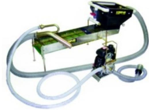
**Keene HBCK25 2.5 Inch Highbanker-Dredge With Honda 2.5HP Engine**
