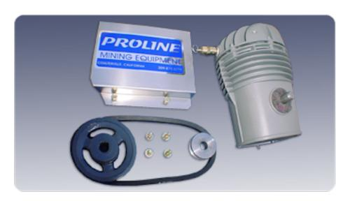
It connects easily to dredge motor to supply hookah breathing system. The T80 compressors are recommended for shallow diving conditions including dredging. Factory recommended RPM is  $1800\ 5/8$ ″ shaft. Produces  $1.8\ CFM$  at  $45\ PSI$ .
