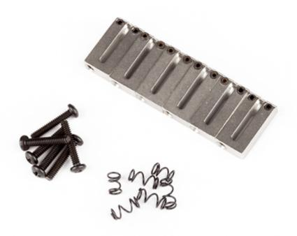
Set of six plated steel bridge saddles with offset intonation screws, for use on American and American Standard series guitars manufactured from 1986-2007. Intonation springs and mounting hardware included. Note that saddles will not fit vintage-style bridge plates due to offset intonation screw design.
