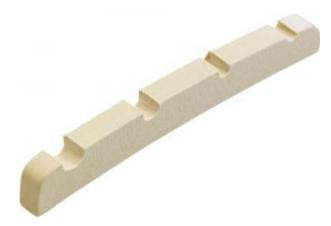
High-quality Micarta (synthetic bone) pre-slotted string nut for use on American Standard Precision Bass and other U.S.-and Mexico-made basses with 9.5"-radius fingerboards. Note that some filing and shaping modifications may be required to ensure proper fit and performance.
