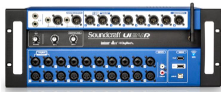
The Soundcraft Ui24R is a complete, rack-mountable, digital mixing and multi-track recording system that delivers flexible
