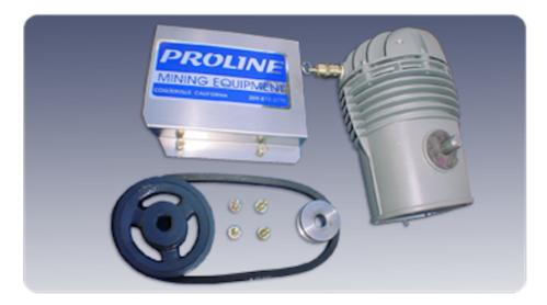
It connects easily to dredge motor to supply hookah breathing system.. The T80 compressors are recommended for shallow diving conditions including dredging. Factory recommended RPM is 1800 5/8" shaft. Produces 1.8 CFM at 45 PSI.
