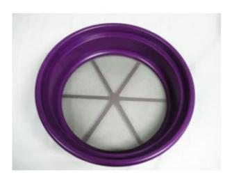
These quality stainless steel classifiers have rugged plastic bodies with stainless steel screens. They are 12 inches wide at the top and are tapered to fit in the top of a 5 gallon bucket. The overall height is 3 1/2 inches and designed to allow for 4 of the classifiers to be nested with an overall height of only 8 1/4 inches. They are easy to use and a must for proper fine gold recovery.
