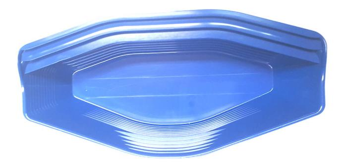
The Gold Claw is very simple to use and the entire process is done under water. Just shake vigorously side to side allowing the gold to settle to the bottom of the pan. Then shake softer while slowly tilting the pan, letting the lighter material fall out of the pan over the large riffles. When down to the heavy concentrates in the pan, transfer the material to the opposite side of the pan and repeat the process till clean gold can be removed from the pan with a snuffer bottle.
