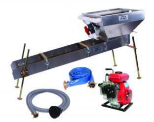
The GOLD BUDDY Highbanker Hopper is attached to the sluice using the GOLD BUDDY Header Adapter making the entire sluice about 4 feet long. Powered by a JOBE 2 1/2 hp, 4-cycle, gasoline pump. The unit can also be set up with a recovery tub to complete a Highbanker recirculating system. Includes 8 feet of 1 1/2 inch intake hose, an intake screen, 25 feet of 1 1/2 inch lay-flat discharge hose, and all necessary fittings.
