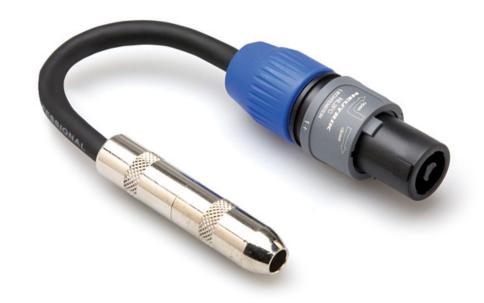
Hosa GSK-116 Speaker Adaptor with Neutrik Speakon Connector on One End and 1/4" Female on the Other. 16AWG, Approximately 6 inches long.
