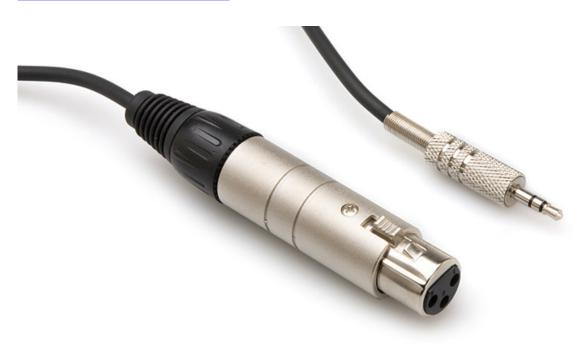
Hosa MIT-156 Line Matching Transformer. 600ohm Low-Z to 2500ohm Medium-Z. Matches microphones with XLR connectors to 3.5mm inputs found on Personal Portable Recording Devices, Camcorders, and Computers.
