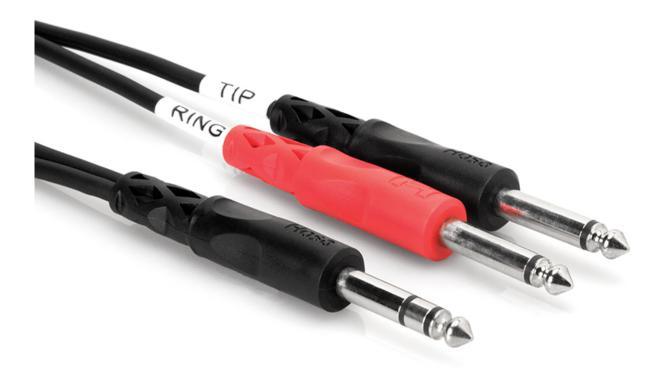
Hosa STP-204 Single 1/4" TRS to Two 1/4" TS. From Mixer's Channel Insert Point to the In and Out of a 1/4"-equipped piece of outboard gear.
