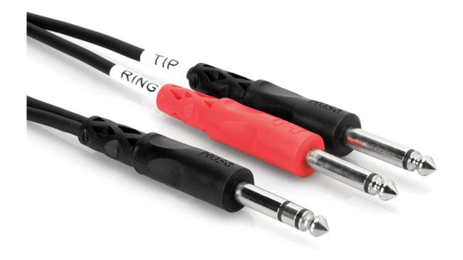
Hosa STP-204 Single  $1/4^{\prime\prime}$  TRS to Two  $1/4^{\prime\prime}$  TS. From Mixer's Channel Insert Point to the In and Out of a  $1/4^{\prime\prime}$ -equipped piece of outboard gear.
