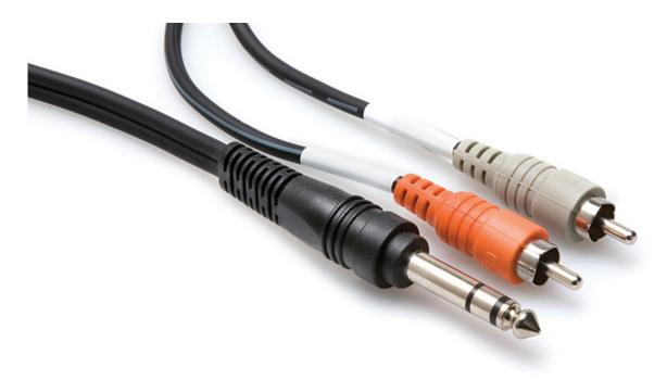
Hosa TRS-204 Single 1/4" TRS to Two RCA. From Mixer's Channel Insert Point to the In and Out of a RCA-equipped piece of outboard gear.
