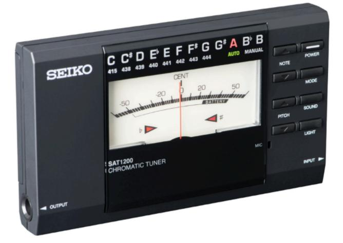
Tuning Range Sound Generation Pitch Shift Terminal A0 – C8 C4 – B4 (1 octave) A4=415, 438- 444Hz (1Hz step) Built-in Microphone Input-Jack, Output-Jack
