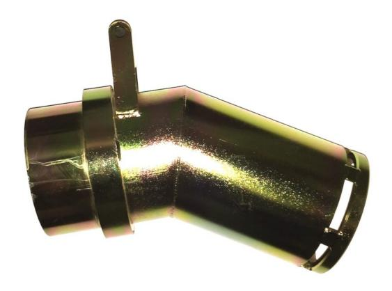
Proline's unique swivel seal is less prone to seizing from sand than other designs. The tip includes a high carbon steel wear ring which is spaced out from the nozzle body to increase dredge capacity and to make it easier to remove large rocks from the tip. This nozzle is built to last!
