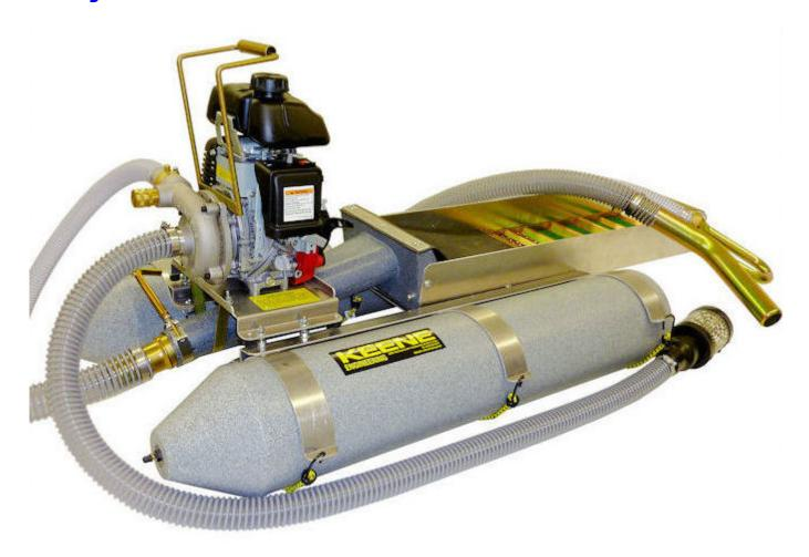
This engine and pump combination produces an unbelievable 100 gallons per minute and up to 160 feet of head pressure. The sluice box is specifically engineered for fine gold recovery and easy clean up. The Model 2004 is constructed with an aluminum frame and is supported with grey hard Marlex pontoons. The model 2004 comes equipped with a suction nozzle.
