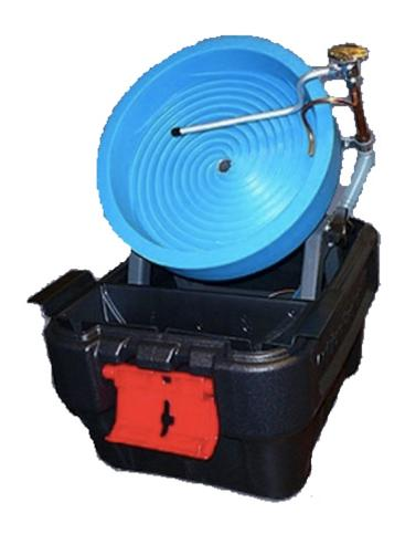
While the Desert Fox Automatic Gold Panning Machine is mainly a finishing machine used in conjunction with a sluice box or other concentrator, you can also use it to prospect for gold. Simply set up the machine and take a few samples systematically and observe which samples contain the most color. Set up your concentrating equipment near the test area with the best show of gold.
