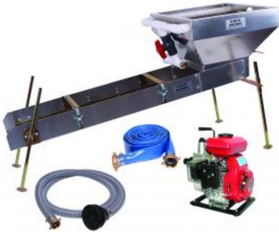
The GOLD BUDDY Highbanker Hopper is attached to the sluice using the GOLD BUDDY Header Adapter making the entire sluice about 4 feet long. Powered by a JOBE 2 1/2 hp, 4-cycle, gasoline pump. The unit can also be set up with a recovery tub to complete a Highbanker recirculating system. Includes 8 feet of 1 1/2 inch intake hose, an intake screen, 25 feet of 1 1/2 inch lay-flat discharge hose, and all necessary fittings.
