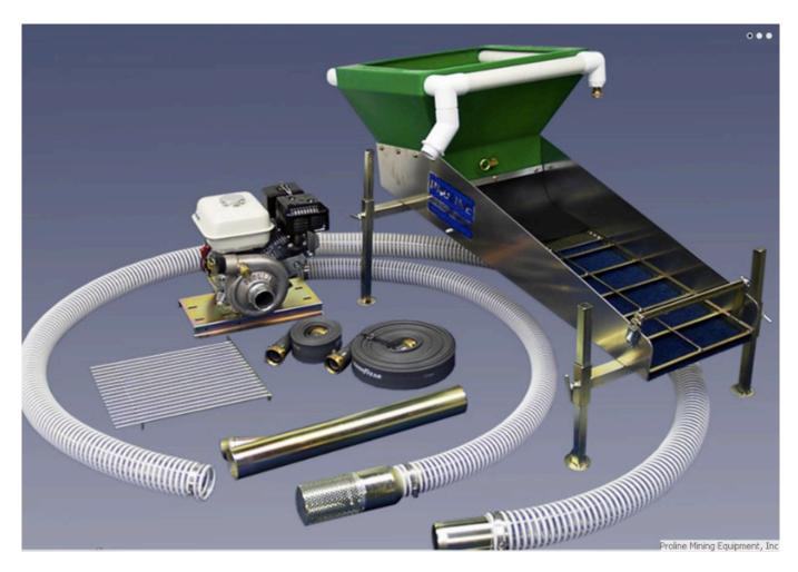
The two triple row spray bars ensure that all of the gravel, clay, roots, etc. are thoroughly washed and separated before running through the recovery system. The grizzly is designed to be strong yet surprisingly lightweight. Like all of our other grizzly's, it is removable to allow for easy access to the classifier and black "V" ribbed matting for inspection and/or cleanup. Also, if the combo is going to be operated solely as a gold dredge, the grizzly can be removed to save weight.
