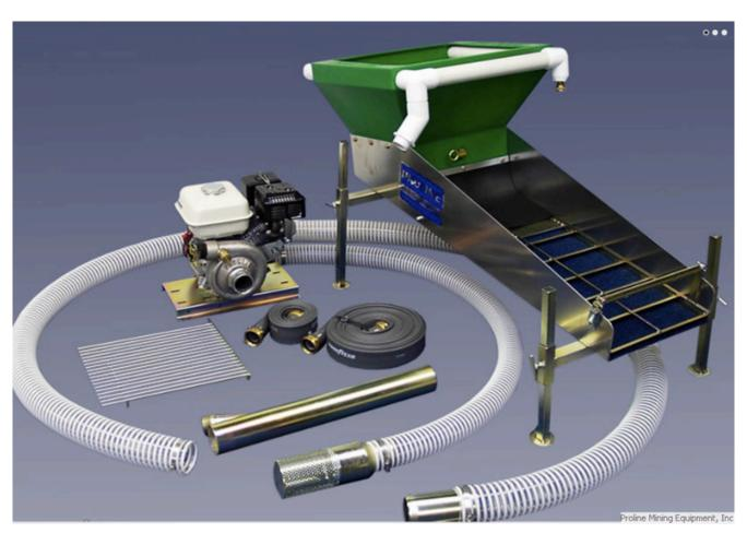
The two triple row spray bars ensure that all of the gravel, clay, roots, etc. are thoroughly washed and separated before
