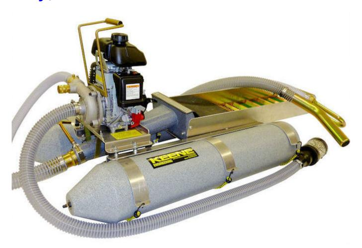
This engine and pump combination produces an unbelievable 100 gallons per minute and up to 160 feet of head pressure. The sluice box is specifically engineered for fine gold recovery and easy clean up. The Model 2004 is constructed with an aluminum frame and is supported with grey hard Marlex
