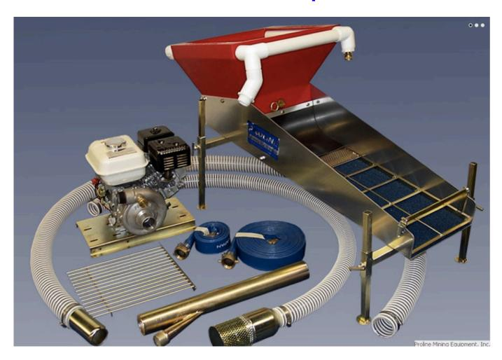
This combo falls halfway in size between the 2" and 3" models and has incorporated some features from both of them. For example, the stand and legs are longer, but made out of the same size material as the 2" combo for weight savings. The polyethylene plastic hopper has been reinforced just like the 3" unit, and the riffles have a stiffening rod on them to ensure a longer life
