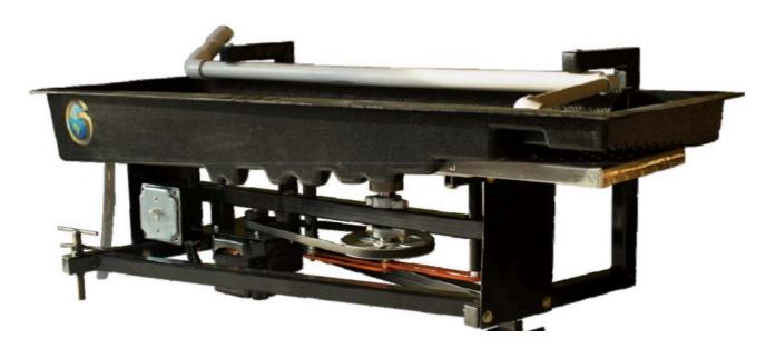
The patented RP-4 is designed for separation of heavy mineral and gemstone concentrate. The RP-4 can process up to 400 lbs. per hour of black sand magnetite or pulverized rock with little to no losses. The RP-4 uses a unique reverse polarity of rare earth magnets, which will cause the magnetite to rise and be washed off into the tails. This allows the micron gold to be released from the magnetite, letting the gold traveling to the catch.
