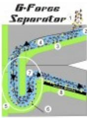
8 mesh minus Gold bearing material 1 is added to the water flow 2 on the slick plate 3. The slurry 4 drops into the G-Force Separator 5. The slurry accelerates around the bottom of the trough and centrifugal force helps move gold outward 6. As all the material leaves the G-Force separator high velocity water comes the lighter material up and away 7. The gold is then dropped into the beginning of the Vortex Mod. 8. This process is repeated in each separation tray.
