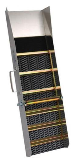
The JOBE 36 is 10 inches wide and 36 inches long weighing only only 8 pounds. The riffles are designed for superior recovery under different water and gravel conditions. The first few riffles are stream riffles to make it easier for the water to start to move the material, followed by Hungarian riffles to enhance recovery if greater stream volume is available. Each sluice includes a section of ribbed black rubber matting for instant gold recognition. A
