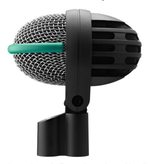
The D112 MkII can handle more than 160 dB SPL without distortion. Its large diaphragm has a very low resonance frequency that delivers a solid and powerful response below 100 Hz. Its authoritative low end is complemented by a narrow-band presence boost at 4 kHz that punches through even dense mixes
